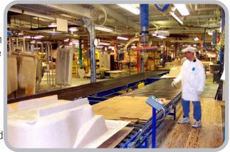
The conveyor system eliminated the need for bulky carts and the chain transfers increased the amount of tubs that can be processed simultaneously. Another concern was aesthetics so they wanted the conveyor painted to match their corporate colors. Conveyer & Caster was able to accomplish this with a powder-based paint by Tiger Dry-Lac.
