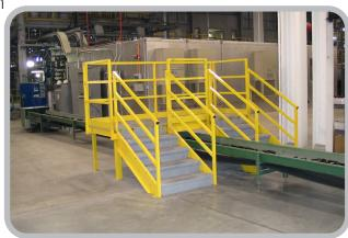
Our engineers started with a steel substructure to support 150 pounds per square foot load capacity. Polyurethane coated plywood was used as the walking surface, to provide a durable, easily cleaned and comfortable work surface. The modular handrail and kickplate assemblies were designed to fit tightly to the poly-plywood floor, creating a barrier to eliminate small objects from falling on to the conveyor and into the bottles
