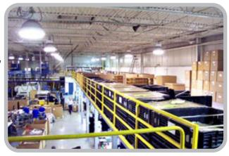
The storage structure utilizes I-Beam construction and a steel checkered plate floor surface. This design allows CDI to store 3,000 pound pallets above the assembly area and move them easily with a manual pallet truck. Access to the mezzanine is done with forklifts, utilizing lift out handrails on the mezzanine floor.
