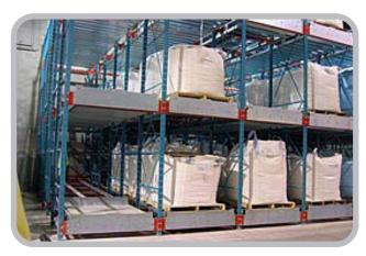
It was determined that the best way to maximize capacity and handle the variety of loads was to engineer, provide and install a Speedrack Modular Rollback® System. Rollback modules are gravity operated, loaded from the front and the loads are pushed back on precision wheeled carts. The patented wheel design and solid steel deck carts handle all of the different load sizes, as well as different weight capacities within the same lane.
