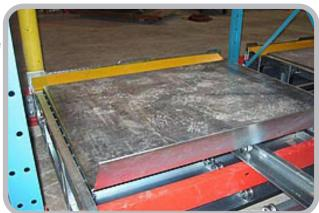
The Modular Rollback® System now holds PBP's raw materials in 70% less space than conventional pallet rack and requires no special lifting equipment or electrical devices.
